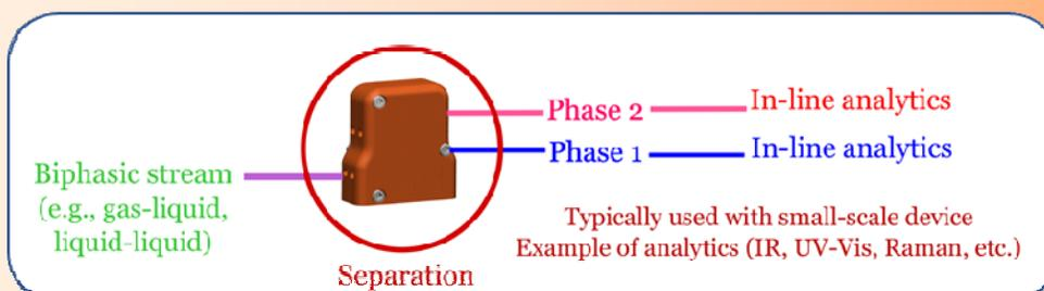
Separation of bi-phasic systems with a Zaiput device allows direct use of in-line analytical equipment.
