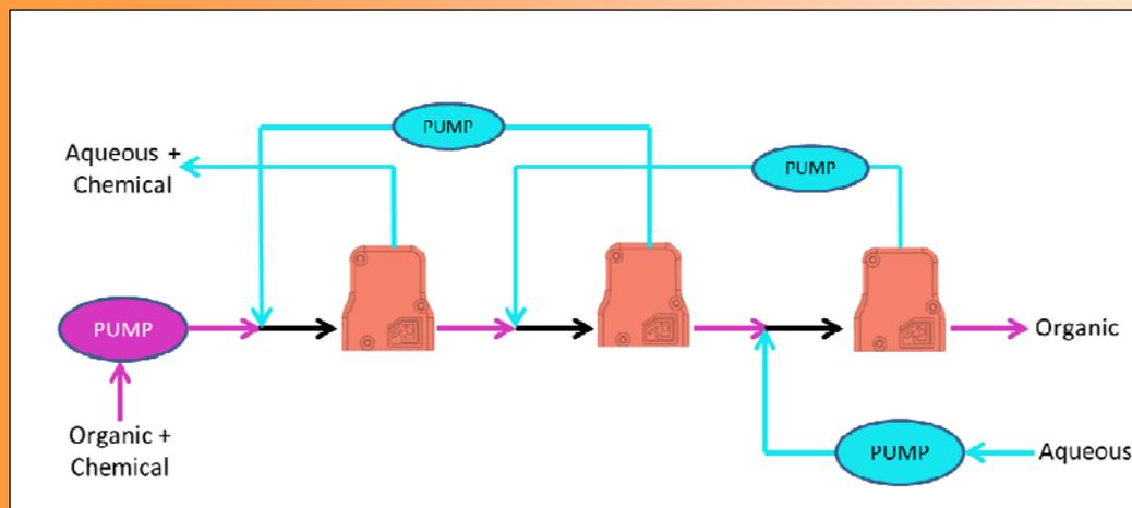
Complex extraction requiring multistage operation can be quickly accomplished.
