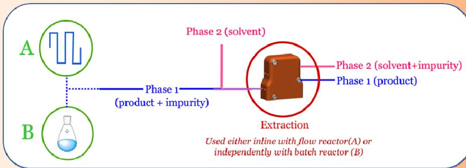
A reaction (in flow or batch) can be followed by a continuous extraction. Advantages are speed, low dead volume, continuous operation and quick separation of emulsions.
