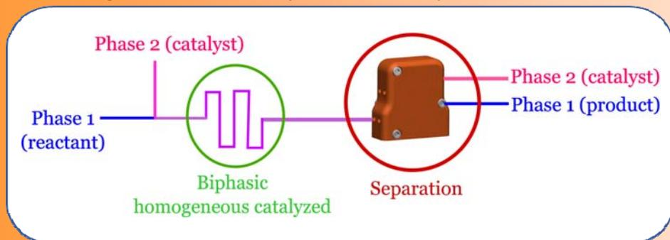
Despite its high selectivity, it is difficult to perform homogeneous catalyst recovery at a large scale because it requires highly active mixing to keep the two liquids in contact. Even at small scale, homogeneous catalysis is rarely used because it poses problems with catalyst recovery via phase separation. Zaiput's separator offers an easy and
