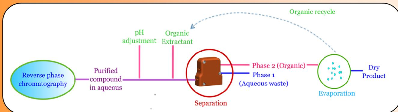
Aqueous work-up for product isolation is tedious and cumbersome, especially in preparative chromatography. In-line single- or multi-stage extraction with a Zaiput device streamlines operation, simplifying solvent recovery.
