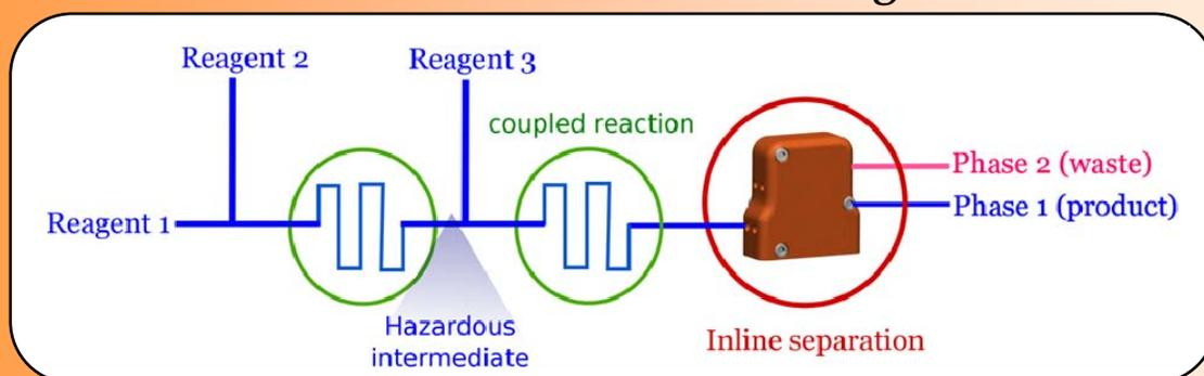
Flow synthesis can be very useful for handling hazardous intermediates because the compounds can be consumed directly into another flow synthesis without isolation.
