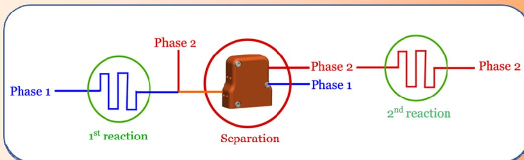
Solvent switching is a common step in multi-step synthesis. In general, it is done manually and in a batchwise process that is slow and tedious.
