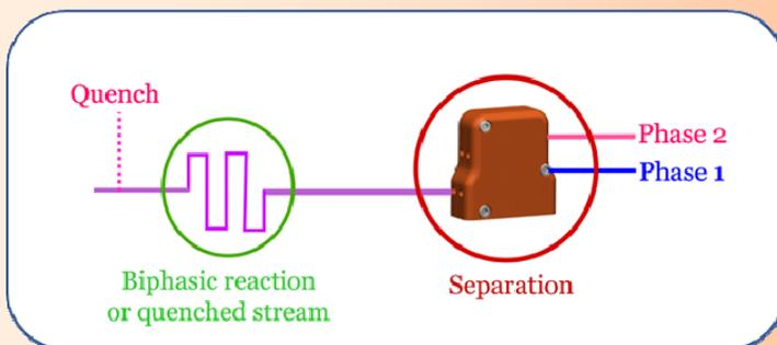
In liquid-liquid reactions, often the reaction stream needs to be quenched by an immiscible phase. Zaiput's liquid-liquid separator can be used downstream or in-line to separate the biphasic reaction.
